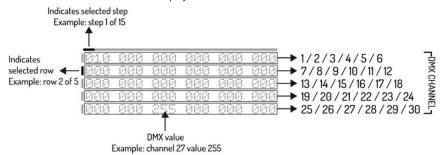
> Select DMX channel with < ▼ > button and select DMX value with the fader corresponding to the DMX channel,
